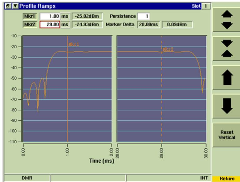
Fig. 2-18 Power Profile Ramps - Adjust Vertical Soft Keys Sub-menu
