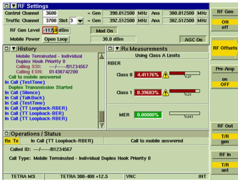
Fig. 5-9 TETRA MS Rx Measurements Tile - Minimized View
