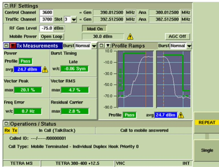
Fig. 5-6 TETRA MS Tx Measurement Tile - Minimized View
