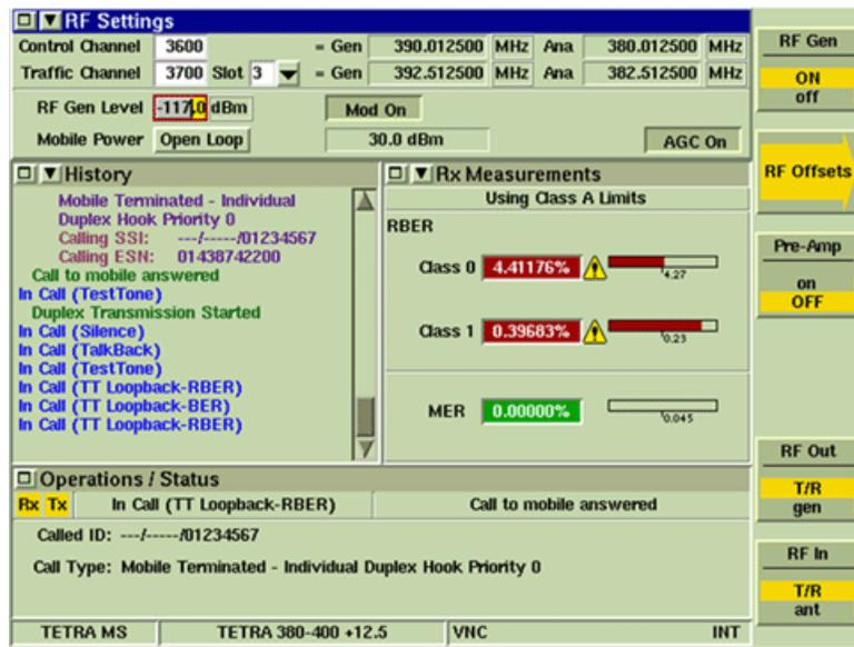
Fig. 4-22 TETRA MS Rx Measurement Tile - Example Limits Shown
