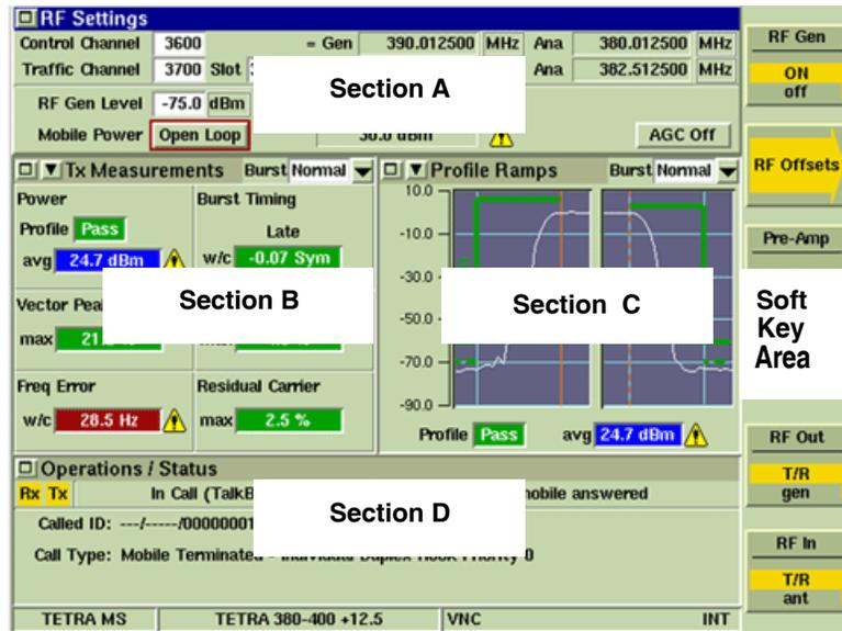
Fig. 5-1 TETRA MS System Display - Tiles Minimized View
