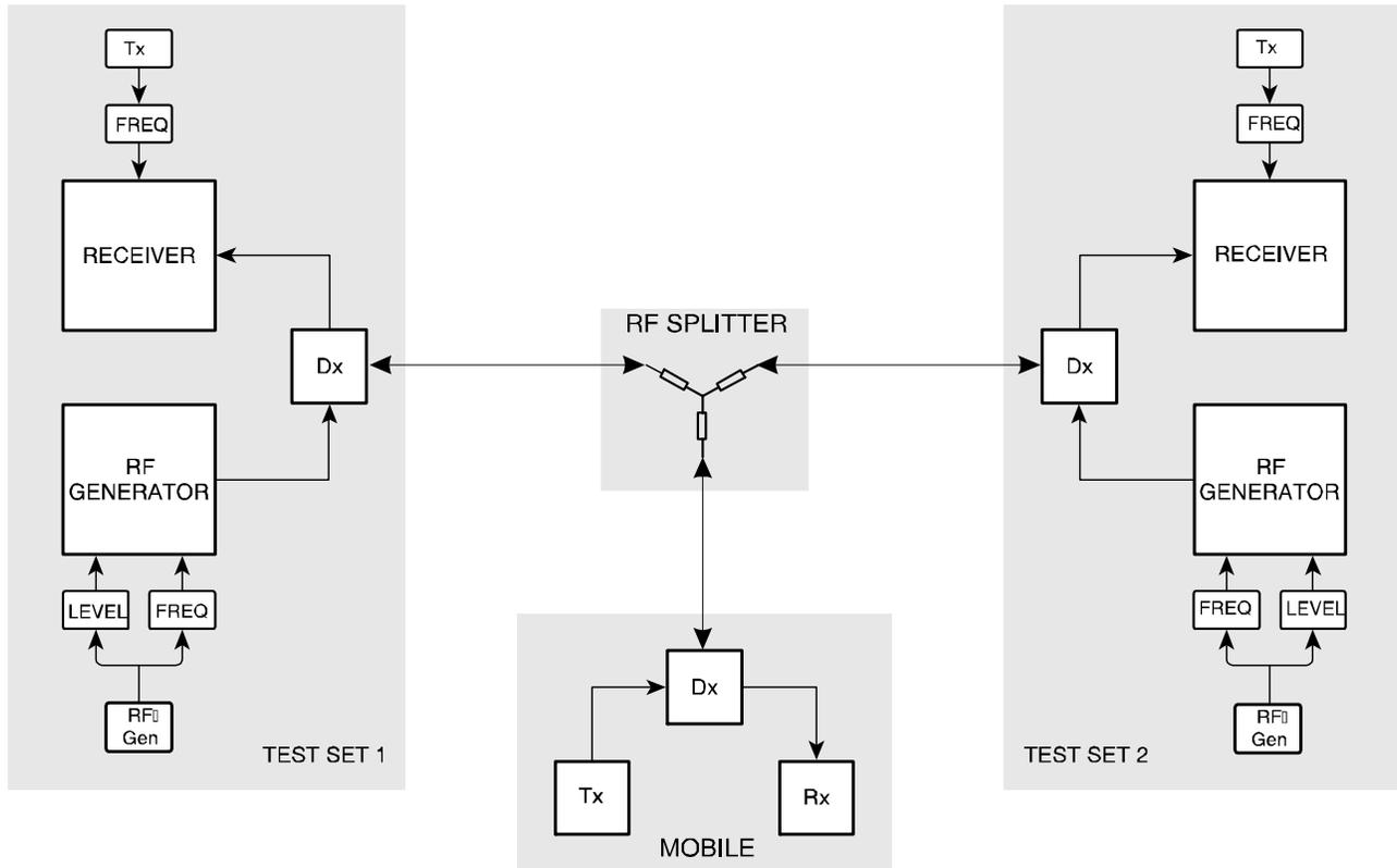
Fig. 5-44 Cell Re-selection Radio Test Set-up
