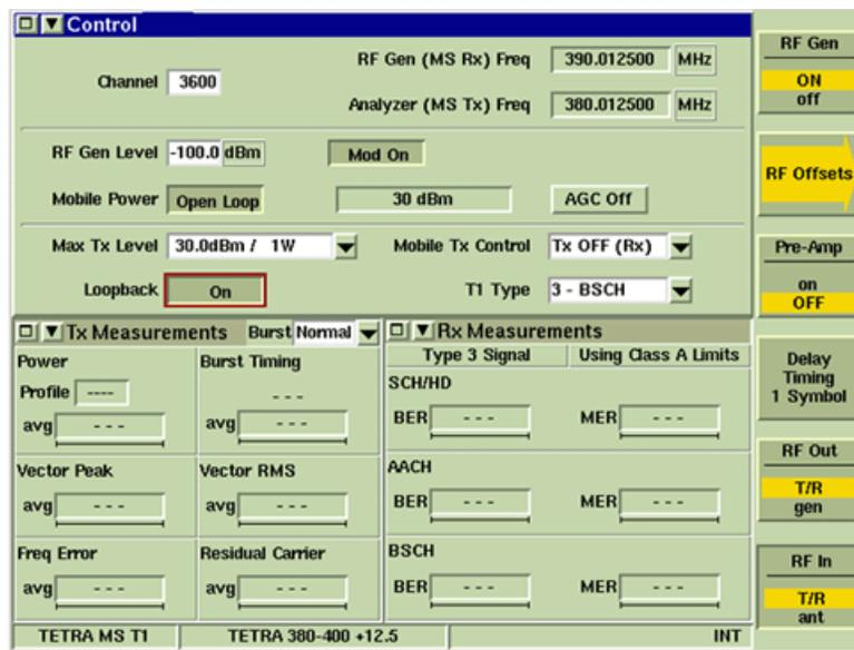
Fig. 6-6 TETRA MS T1 Rx Measurements Tile - Minimized View (Loopback ON)
