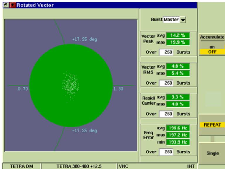
Fig. 9-16 TETRA DM Rotate Vector Tile - Accumulate ON
