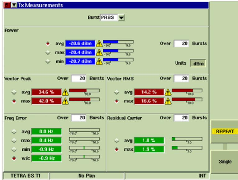
Fig. 8-10 TETRA BS T1 Tx Measurements Tile - Maximized View
