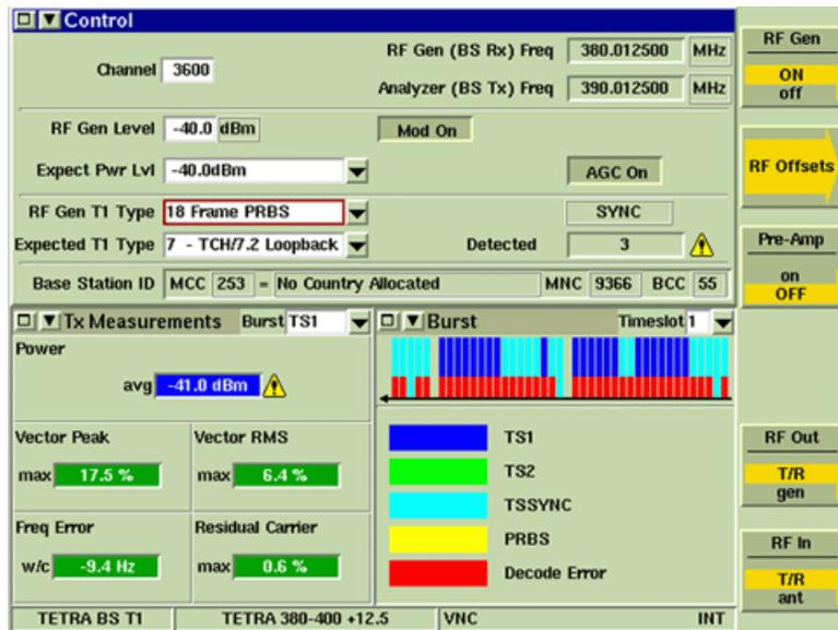
Fig. 8-8 TETRA BS T1 - Burst Tile Measurements Tile location
