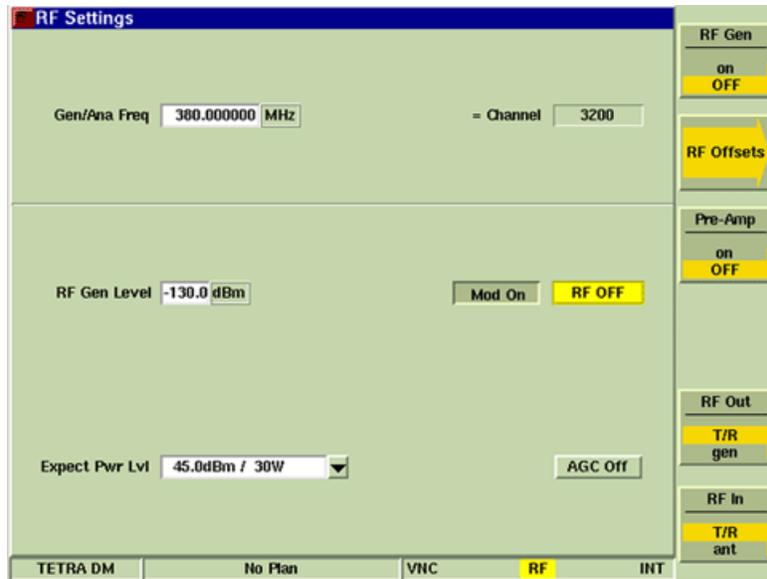
Fig. 9-3 TETRA DM RF Settings Tile - No Channel Plan Selected
