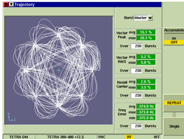
Fig. 9-14 TETRA DM Trajectory Tile - Maximized View
