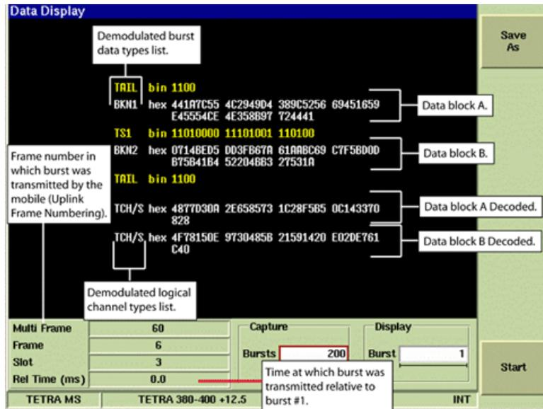
Fig. 2-11 TETRA MS Data Display Tile with Captured Data Bursts
