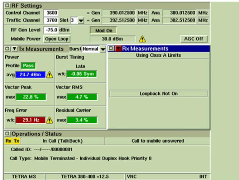
Fig. 5-8 TETRA MS Rx Measurements Tile - Loopback OFF
