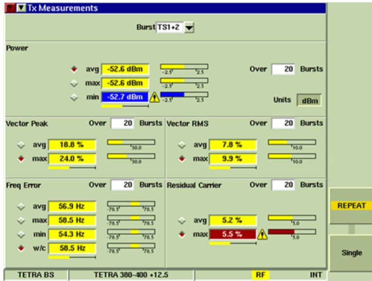
Fig. 7-6 TETRA BS Tx Measurements Tile - Maximized View
