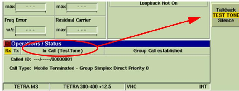
Fig. 5-46 Audio Test - Test Tone Selected
