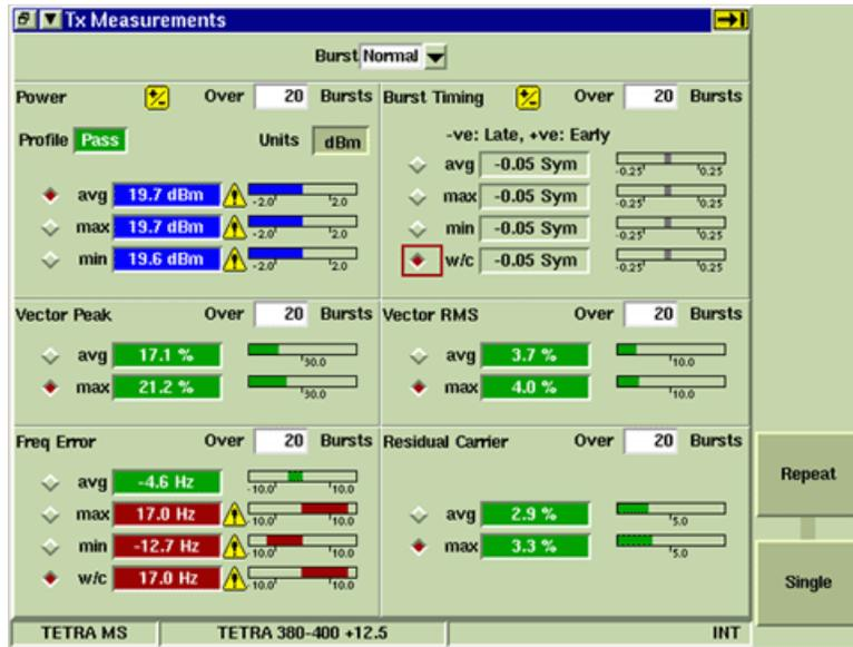
Fig. 5-7 TETRA MS Tx Measurement Tile - Maximized View
