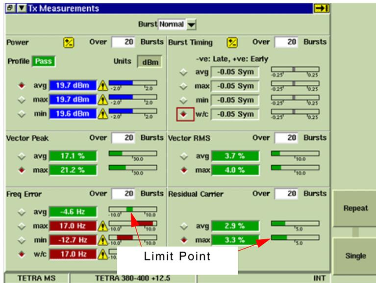
Fig. 4-18 TETRA MS Tx Measurements Tile - Limit Points Shown
